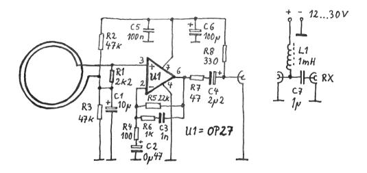
Figure 2. Circuit diagram of the loop amplifier
