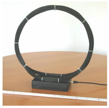
Figure 1. The prototype loop has 40 turns and a diameter of 38 cm.
